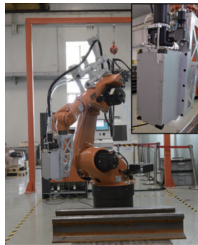
图1 钢轨激光强化设备 Fig. 1 Laser hardening device of rail
